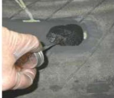
Brushing the cement both into the cleaned area and the surface of the gray gum on the patch.
