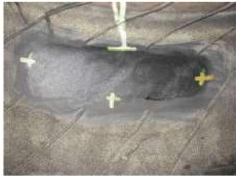
Allowing the solvent to dry 5min-10min after brushing the cement, (depending on temperature).
