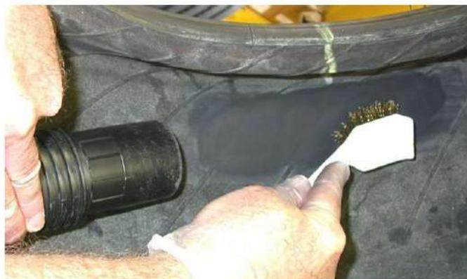
Using a brass-bristle brush and cleaner to remove buffing dust from the buffed area.
